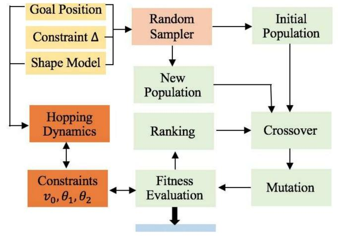
Schematic of the optimized path planner using Evolutionary Algorithm. Credit: Kalita & Thangavelautham.
